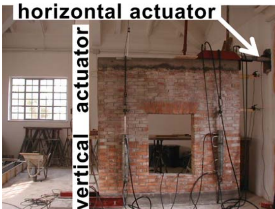
Fig. 9 Loading system: actuators and steel reaction frame
