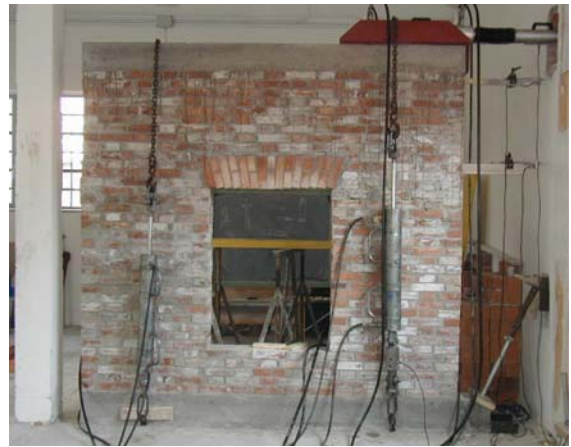
Fig. 4 Test perforated wall; texture 2 and test setup
