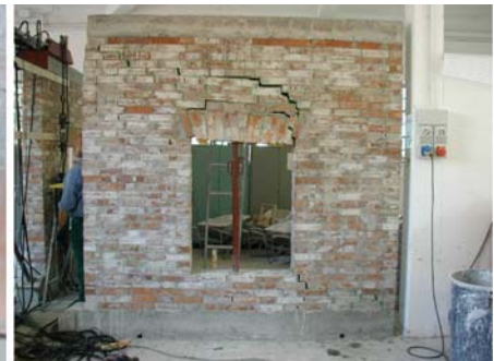
Fig. 7 Test rig; concrete braced loading distribution beams
