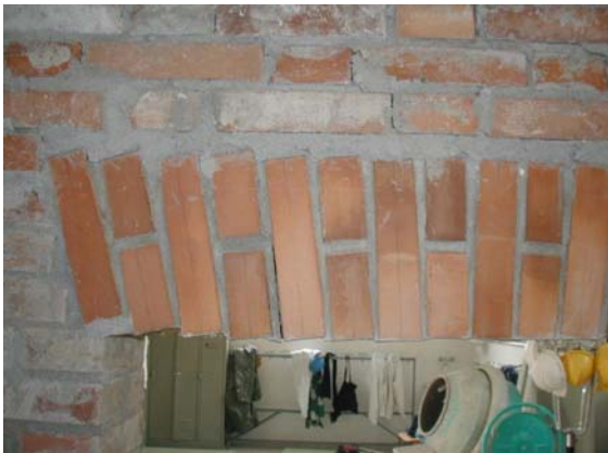
Fig. 6 Closeup of the lintel beam during test 1–3, at an overall drift level of about 1.3%
