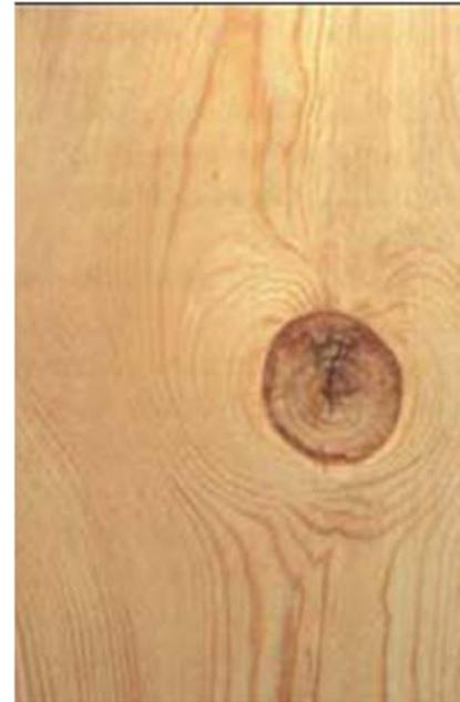
Sawn timber beam with knots
