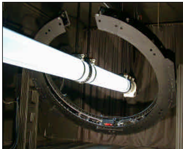
fig. 2: First goniophotometer for measuring the spatial light distribution of various hollow light guides (TUB, Berlin).
